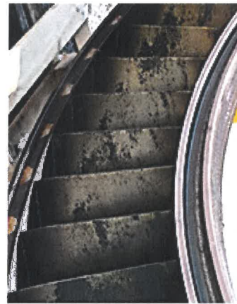
GT2, 4th stage vane, pressure side On-line cleaned with Cleaner A Off-line cleaned with TURBOTECT 2020
